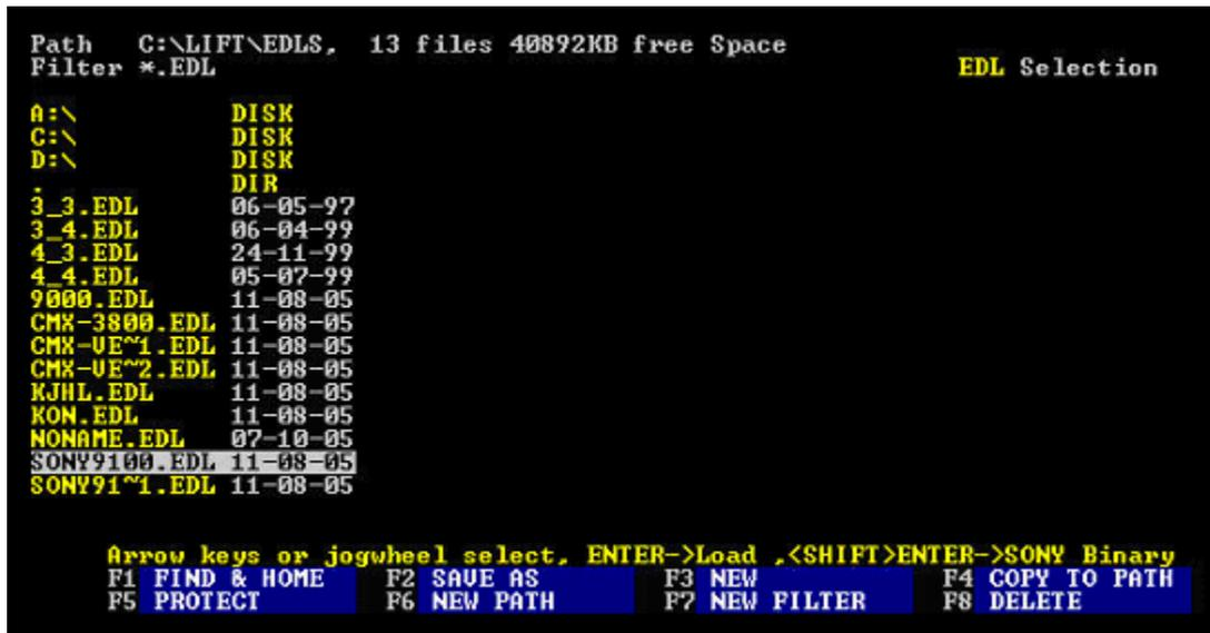
2. Select a file from the displayed list. To move the **selection bar**, turn the jog knob, use the **[←]** and **[→]** arrow keys, or use the **[HOME]**, **[PGUP]**, **[PGDN]** and **[END]** functions in the numeric keypad to select the desired file.
